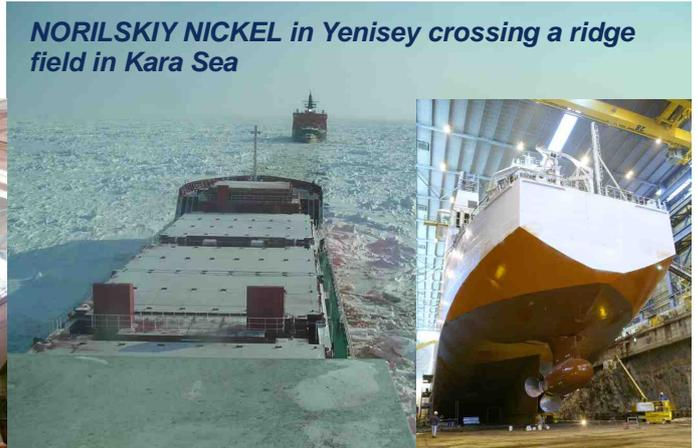
The container vessel MS Norilskiy Nickel is designed to operate independently without icebreaker assistance carrying mining products from Dudinka (Yenisey River, Russia) to the market, mainly to Murmansk.
