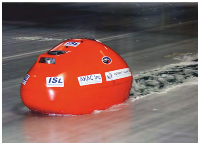
ISL model making forward progress in 15cm Level ice.
