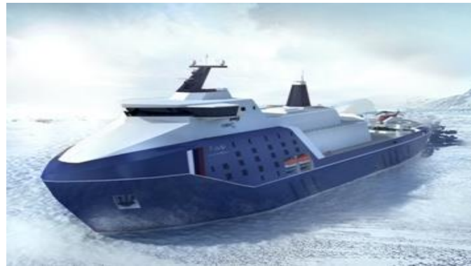
Atomic turbo-electric icebreaker Project 105010 (IB Leader) with the propulsion power of 120 MW
