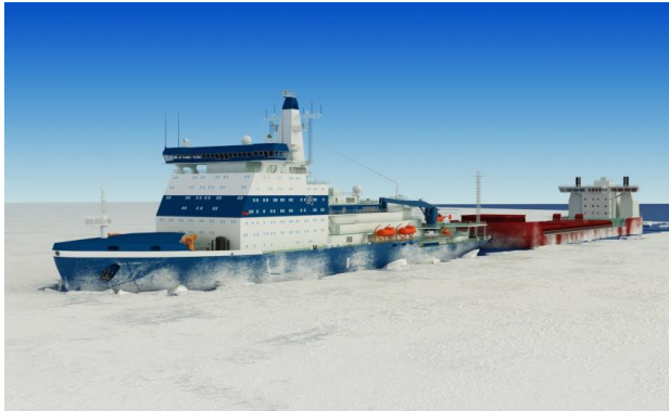
Universal atomic icebreaker Project 22220 (IB60) with the propulsion power of 60 MW
