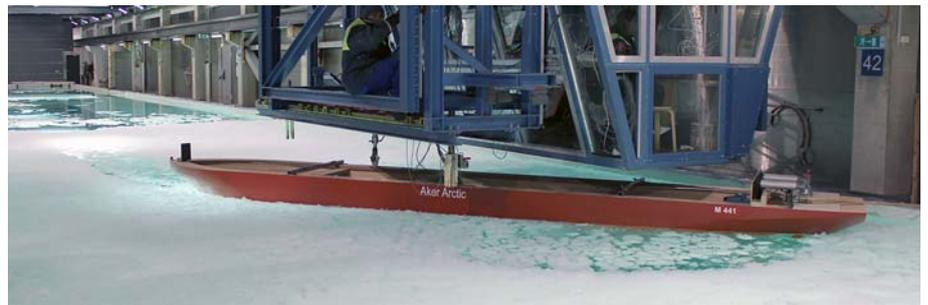
**Aker Arctic has developed an Arctic Condensate Tanker for transporting gas condensate from the Yamal LNG's natural gas fields in the Russian Arctic to customers in Europe and Asia. The Arc7 ice class vessel is based on Aker Arctic's Double Acting Ship (DAS™) principle and it can operate independently in up to 1.8 m thick level ice.**
