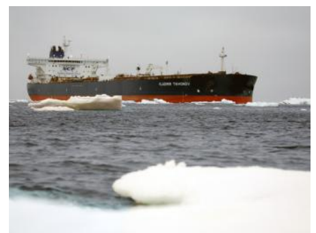
During 2011 a new route North of the New Siberian Islands was established, where the water is deep enough to accommodate tankers with draughts of over 12 metres, and for the first time in history, the route was navigated by the Sovcomflot tanker Vladimir Tikhonov, a Suezmax ice class 1A vessel with a deadweight of over 160.000 tons. ■
