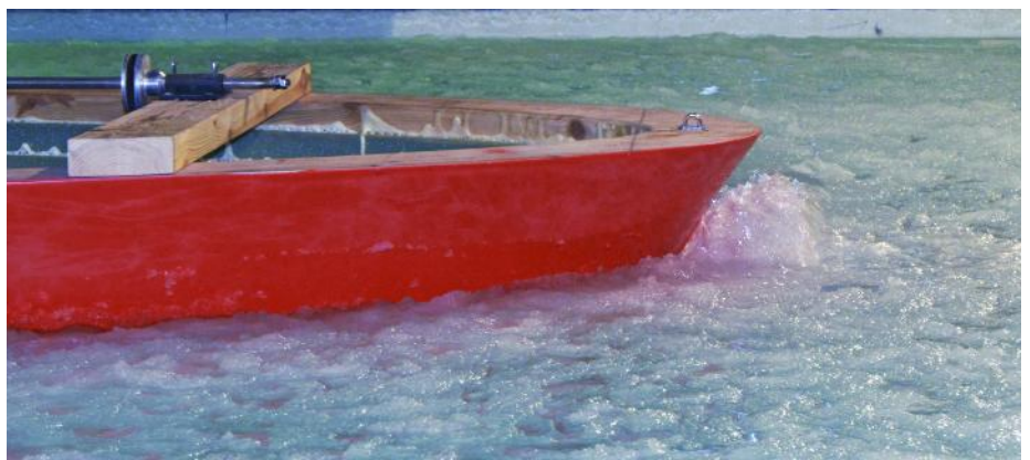
The total power reduction benefit with the help of the vertical thruster system in unfrozen and consolidated channels is up to 20%. The channels are defined by the Finnish-Swedish Ice Class Rules.
