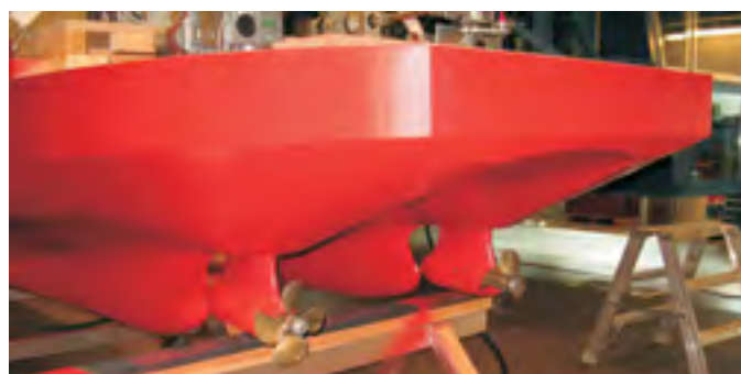
Model ready for astern running ice tests with pulling type pods turned for backing position
