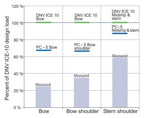
The preliminary results from the Gulf of Bothnia measurements on aft shoulder ice impact show relatively high loads compared to loads measured from other areas. The blue lines show the level of PC 5 and green lines DNV ice-10 dimensioning criteria. The final report may lead to class rule improvements.
