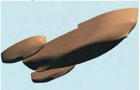
The Trimaran hull used for concept development
