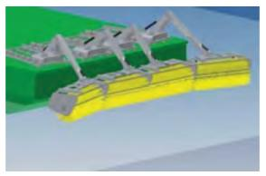
SYKE- developed ice brush skimmer packages that could be a standard outfit for any Arctic support vessel in the future.
