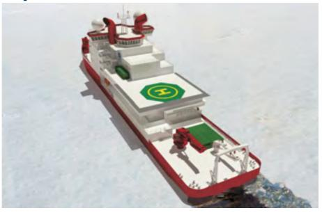
position keeping, two bow tunnel thrusters are provided. The power generation station consists of four main diesel generators sets. Propulsion power is 2 x 7.5 MW and in the aft ship there are two skegs protecting the propulsion machinery from multiyear ice blocks. With one engine the vessel can advance 12 knots, with two engines 15 knots and in ice all four engines are used as needed.
