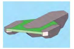
Simplified ship hull used for determining dimensioning loads
