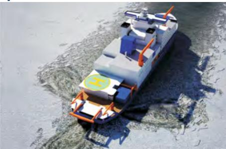
The triple azipod solution enables the possibility to clean the ice around the hull by steering the propeller wake in the needed direction. The solution also effectively prevents ice from going under the bottom, protecting the sensitive science equipment and allowing research work through the moon pool in hard ice conditions.
