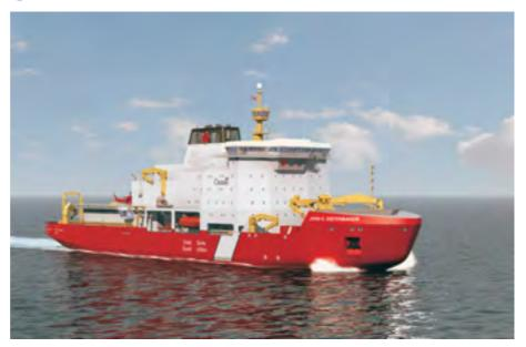
The Canadian polar icebreaker is a step forward for Canada in icebreaker history with an icebreaking performance of 2.5 m level ice with 30 cm snow.
