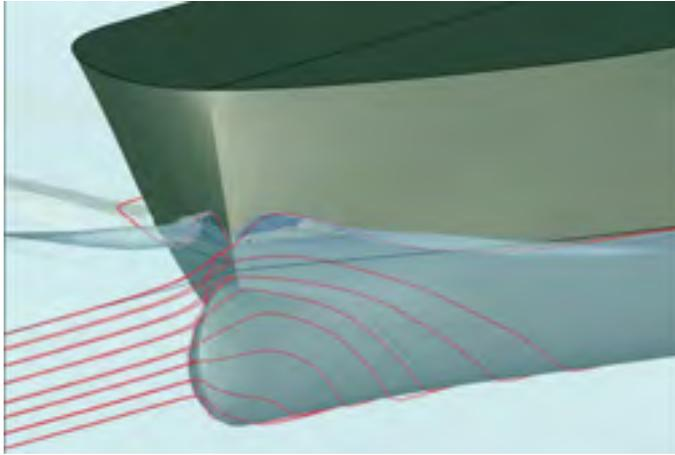
*With the new Computational Fluid Dynamics program more alternatives can be evaluated in detail before open water model tests.*
