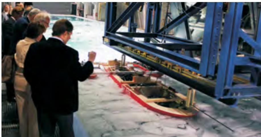
As has been described in the previous issues of Arctic Passion News, AARC is currently developing a trimaran type icebreaker, which could be utilised in escort icebreaking, ice management as well as a deck cargo carrier or an icegoing seismic vessel where the large deck area could be used for higher capacities than in traditional monohull ships.
