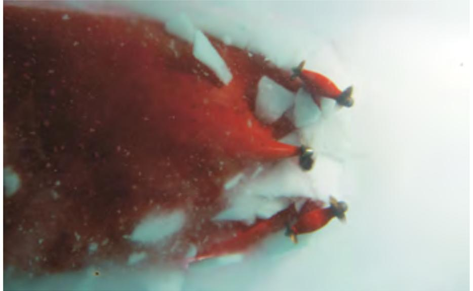
The contra-rotating propellers (CRP) have commonly been used in open water solutions due to their typically higher efficiency, which is very important for any ship designer and operator in the forthcoming days of energy saving goals and emission controls. Aker Arctic and Steerprop decided some time ago to join forces for developing ice capable CRP thruster solutions. Various applications have been brought to initial testing, including solutions for the oblique
