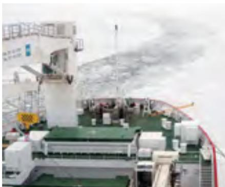
*As a member of the Joint Industry Project, AARC is responsible for the aft shoulder ice load analysis in the ice trials of the newly built research and supply vessel S.A. Agulhas II bringing useful data and knowledge for ice impact loads to the design of new vessels.*
