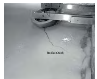
Tests showed that the trimaran breaks ice more efficiently than a conventional ship of the same width, because of the construction with a centre hull and two pontoons on the side.
