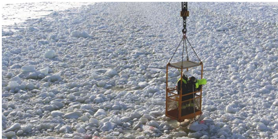
This ice channel close to Kemi stays open all winter, but is filled with brash ice, which was measured 174 cm thick. Polaris managed 14 knots in the channel without any trouble.
