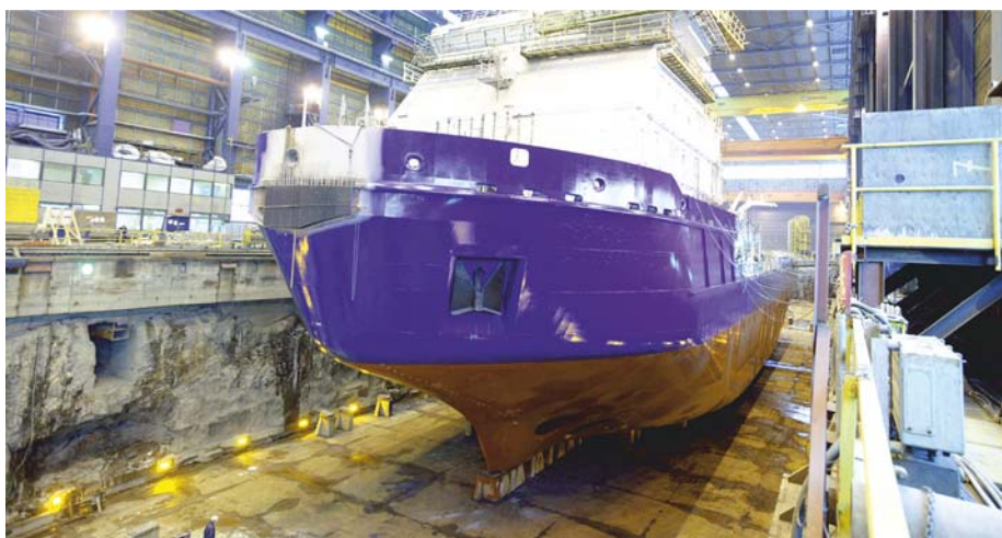
Typical icebreaking bow form
