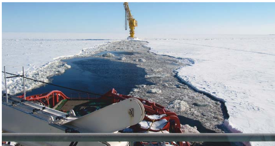
The Baltika clears the loading area by pushing the ice away.
