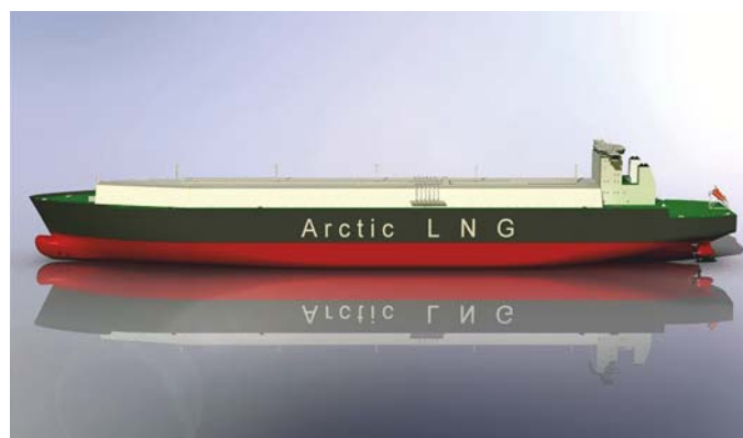
Alternative design with the GTT No-96 tanks with a large capacity of 224,000m 3 . The same propulsion principle with three propellers was used.
