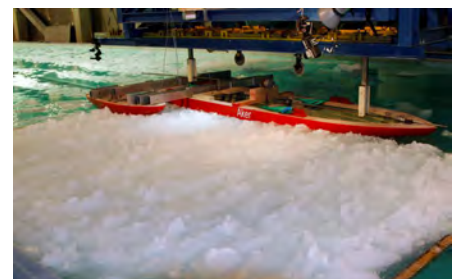
Simplified ship hull was used for determining dimensioning ultimate ice loads.
