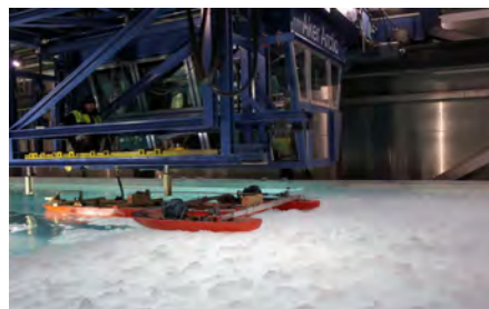
Breaking wide channel in level ice bow ahead.
