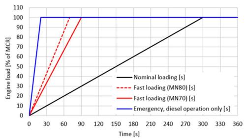
Loading rates Constant speed 31DF engines (DE / Aux / CPP) Normal loading rate, constant speed engines, 720/750 rpm (DE / Aux / CPP) Source: Wärtsilä
