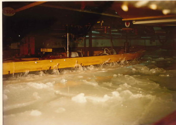
Fig. 18 The model in a ridge with 4000 hp bubbling. Note spray of water.
