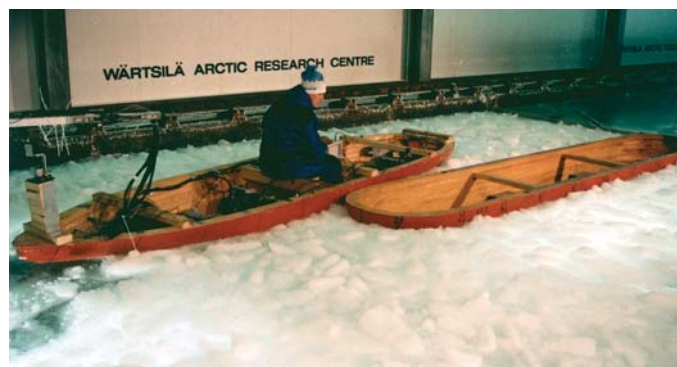
In the 1980s, operational model tests were often conducted by manoeuvring the model manually. Model of icebreaker Otso, assisting another vessel in heavy brash ice, is steered by her future captain, Atso Uusiahho.
