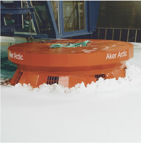
Semi-submersible drilling unit Arctic S was tested both in gravity based (left) and floating (right) mode.
