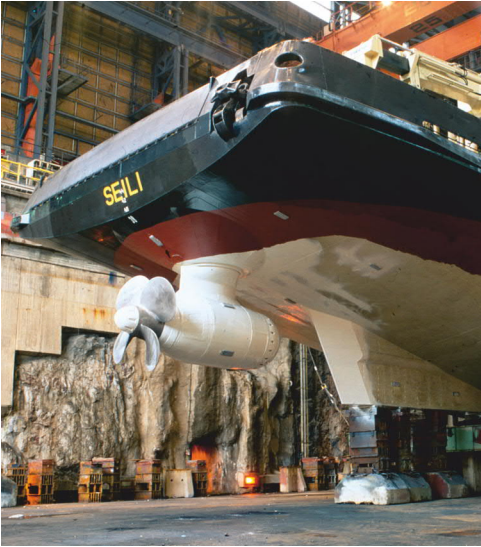
The first Azipod unit was installed to fairway supply vessel Seili.
