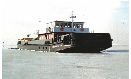
River icebreaker Röthelstein, breaking ice and pushing barges on the Danube river.
