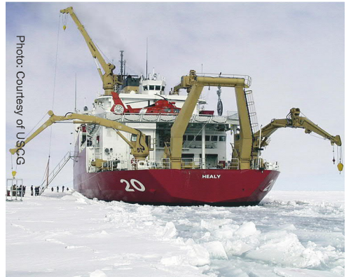
USCGC Healy is the United States' largest and most technologically advanced icebreaker. Hull form development and propulsion line engineering by MARC were based on the Finnish diesel-electric icebreaker Otso.
