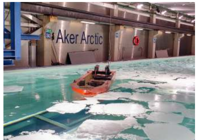
A DP controlled model fending off ice floes coming its way
