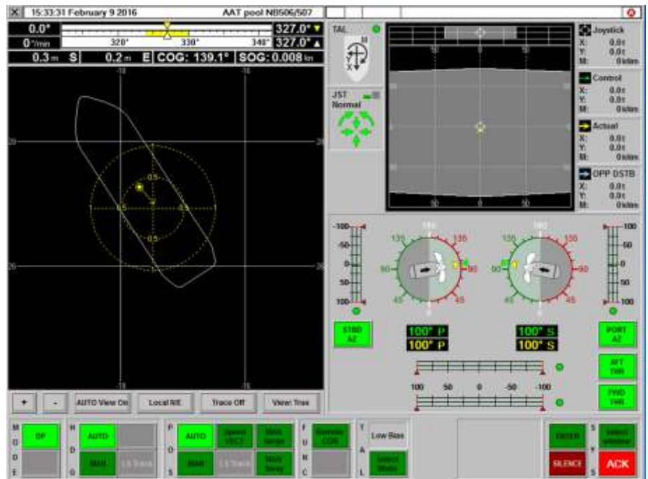
A view of the DP control station.
