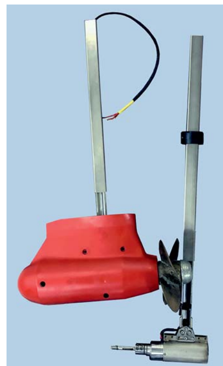
New propulsion units for model testing have been developed.
