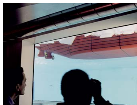
A wireless system allows complete free manoeuvrability of the models.
