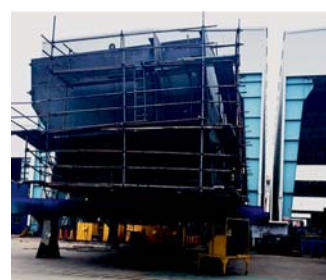
The steel hull is being welded at Jiangnan Shipyard in Shanghai.
