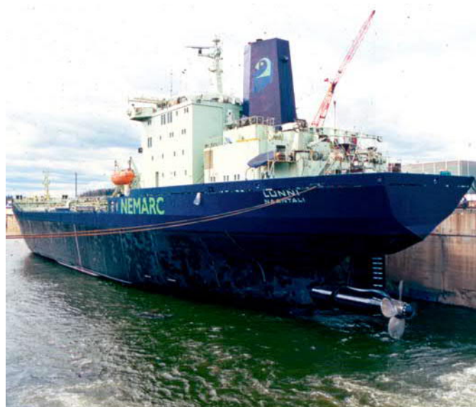
The real breakthrough for the Azipod, and the DAS™ concept, occurred with the conversions of the ice-going tankers Uikku (1993) and Lunni (1994).
