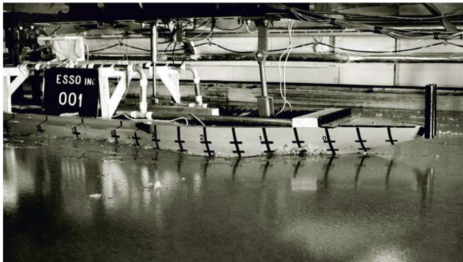
The first ever ice model test conducted in Finland was a resistance test in level ice of SS Manhattan.
