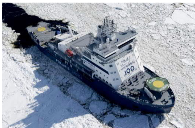
Polaris, built in 2016, is the most powerful icebreaker ever to fly the Finnish flag and the first icebreaker in the world to feature environmentally friendly dual-fuel engines capable of using both low-sulphur marine diesel oil (LSMDO) and liquefied natural gas (LNG). It has excellent manoeuvrability due to the two Azipod units in stern and one in bow.
