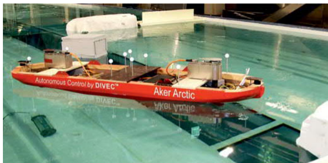
Computer controlled ship model approaching docking on quay represents the future trend in model testing.
