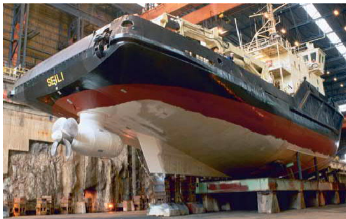
The first Azipod unit was installed to fairway supply vessel Seili.
