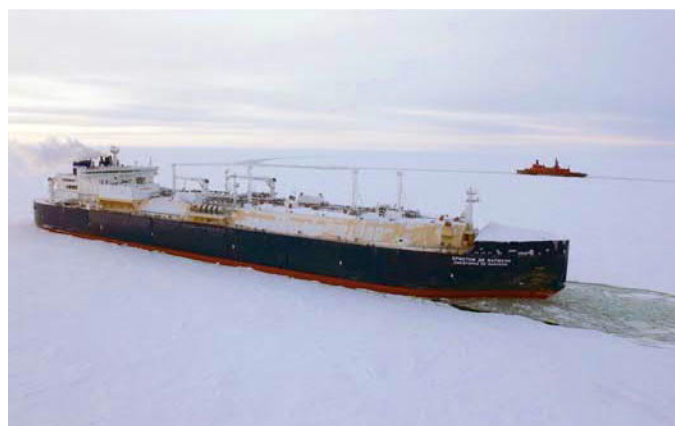
Aker Arctic has been leading the development of Arctic LNG carriers over the years resulting in Yamalmax icebreaking LNG carriers. The vessels are based on the DAS™ concept and capable of operating independently without icebreaker escort along the Northern Sea Route. The hull form has been extensively tested in Aker Arctic's ice model test laboratory. The first Yamalmax carrier, Christophe de Margerie, was delivered in 2016.
