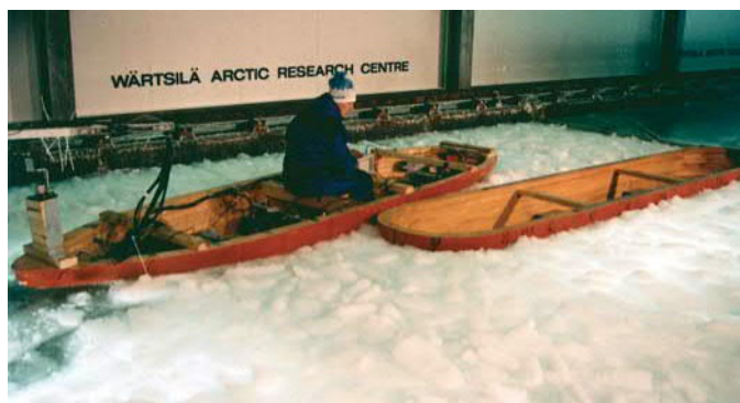
In the 1980s, operational model tests were often conducted by manoeuvring the model manually. Model of icebreaker Otso, assisting another vessel in heavy brash ice, is steered by her future captain, Atso Uusiaho.
