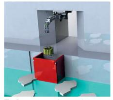
The figure presents the extended position of the sidepool, where the integrated hatches are pushed outwards from the side creating an icefree area at the side. As a result, research equipment and persons can be deployed safely.
