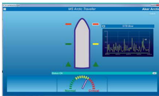
The Ice Load Monitoring System (ILMS) helps the captain to predict ice loads and decide how to proceed in an ice field.
