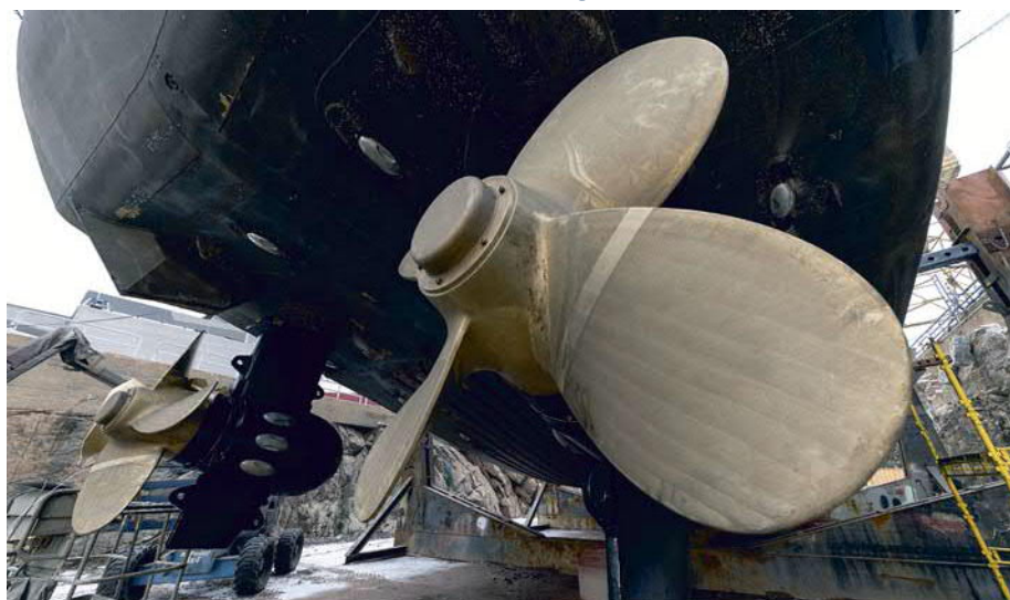
The propellers, based on the results of the development program, have been installed on the Finnish ice class IA ASD tug Calypso .
