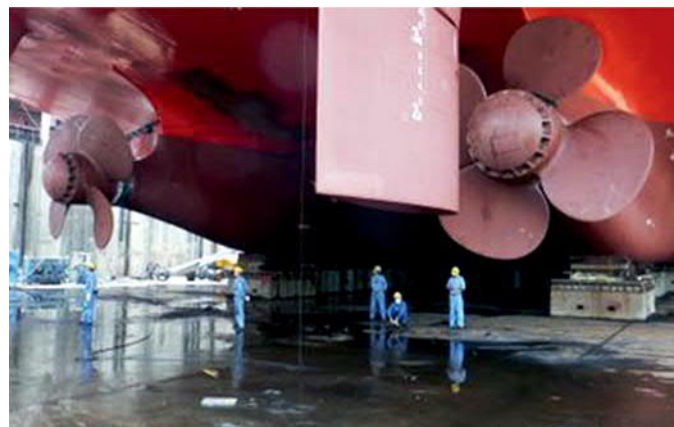
The Aker Arctic designed module carriers Audax and Pugnax are equipped with tailor-made propellers for use in extremely heavy ice conditions.
