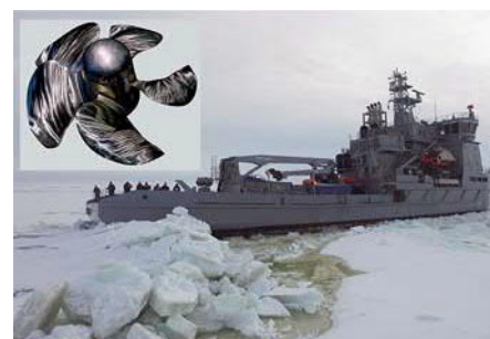
Multipurpose vessel Louhi is equipped with stainless steel propellers, but was fitted with a bronze propeller for ice tests in 2016 and 2017.
