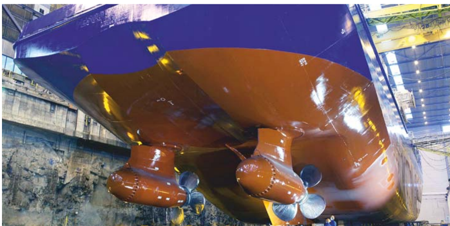
Icebreaking aftship hull form – “double acting ship”
