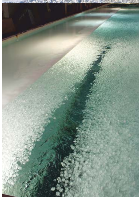
Ice cubes represent a situation where there is no cohesion in the ice. Six m 3 of ice cubes were used for this test.
