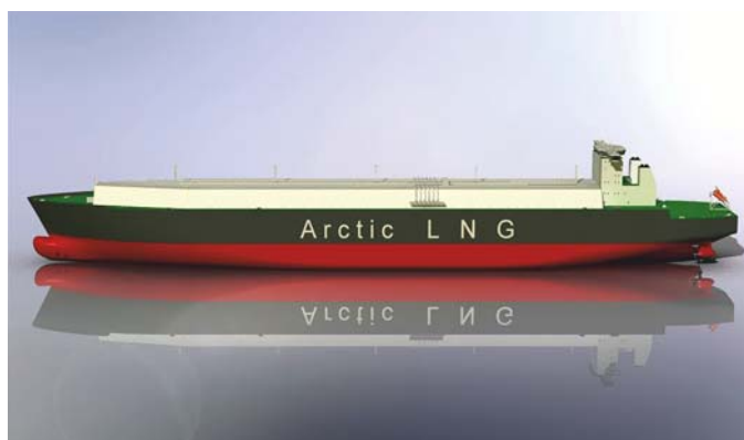
Alternative design with the GTT No-96 tanks with a large capacity of 224,000m³. The same propulsion principle with three propellers was used.
