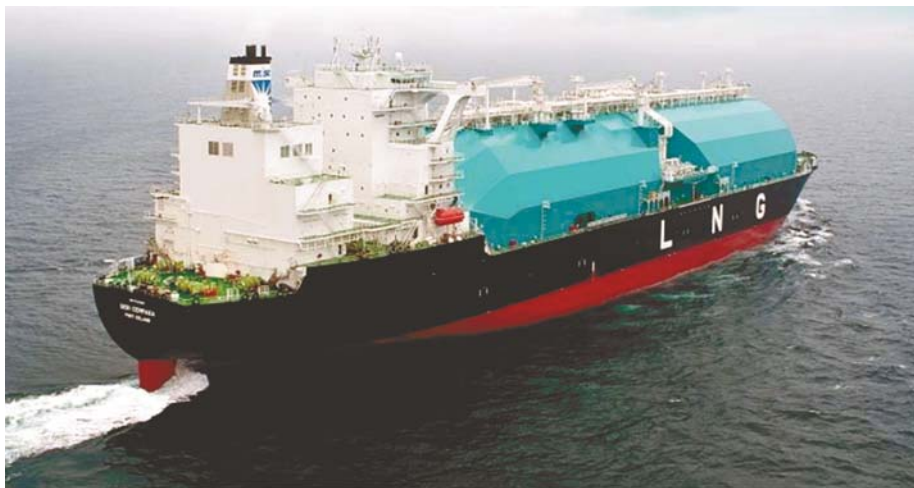
"Seri Campaka" – The third ship in a series of five IHS-Moss type LNG carriers for a Malaysian owner built by Hyundai Heavy Industries. The hull design with its continuous tank cover is based on Aker Arctic's "IHS" concept with improved hull strength and reduced steel weight.
