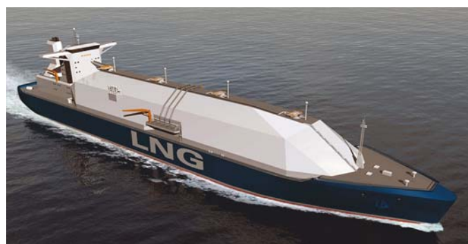
Integrated Hull Structure: Moss cargo tanks are covered by a structurally continuous cover, common to all cargo holds, which improves hull strength.
