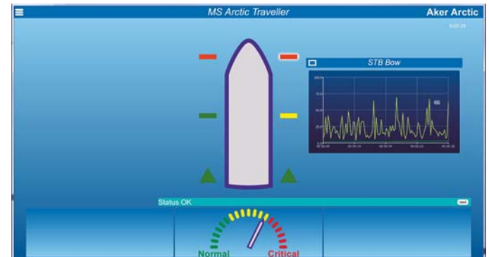
The ice load monitoring system has been operating for two years on icebreaker Baltika.
