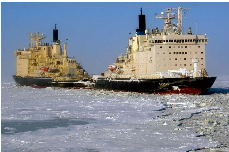
In terms of icebreaking capability, the Aker ARC 130 A design is comparable to the well-known nuclear-powered icebreakers Taymyr and Vaygach, but requires about 40% less propulsion power.
