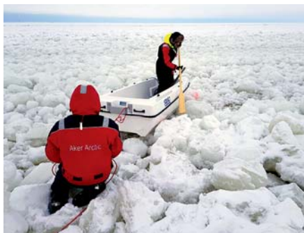
A sledge was acquired which could carry the drilling equipment and also serve as a rescue boat in case someone would fall into the freezing water.
