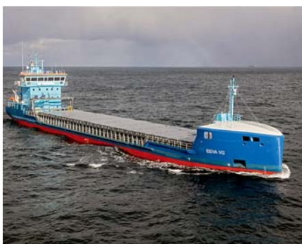
The vessel used for the full-scale test was cargo vessel Eeva VG, owned by Meriaura Ltd. She is a 103-metres-long and 13.6 metres wide dual-fuelled dry cargo carrier based on the VG EcoCoaster design, jointly developed by Meriaura Group, Foreship and Aker Arctic Technology. Ice model tests were performed in Aker Arctic's ice laboratory in Helsinki.
