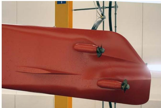
Aker Arctic has developed a new stern design specially intended for ice management vessels. Among many other benefits, the design will improve the flushing effect of the propulsion units compared to a traditional propulsion arrangement. The flushing effect of water flow is typically used in ice management operations to clear ice away to achieve open water areas.
