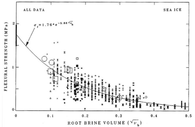
Picture 2. Flexural strength versus the square root of the brine volume for first-year sea ice (Timco and O'Brien, 1994)
