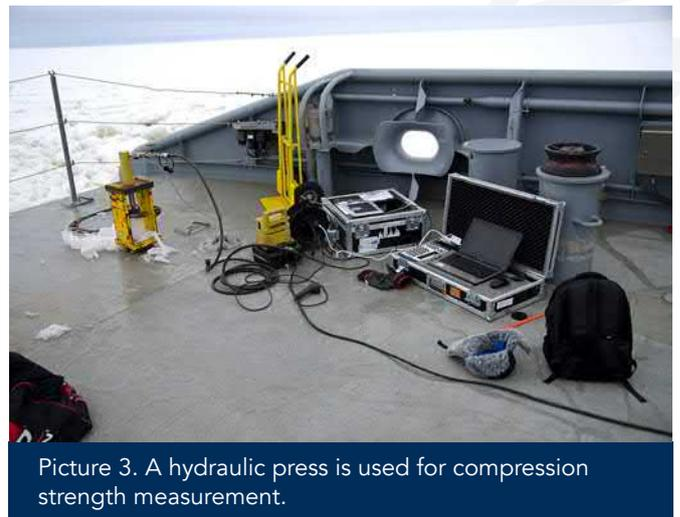
Picture 3. A hydraulic press is used for compression strength measurement.
