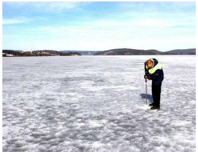
Ice thickness was measured by drilling holes into the ice along the ship track and measuring the thickness with an L-shaped rod.
