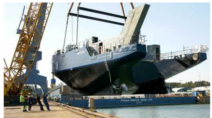
The ILMS will be used to measure the loads at the connection between the bow and the tugboat Calypso , and on the two shaft lines of the detachable bow.
