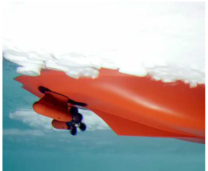
The new vessel concept is fitted with twin azimuth thrusters.
