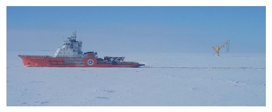
Main purpose of this vessel is support to loading operations at Arctic Gates Terminal, keep ice channel in operate condition during ice season and escort tankers to and away from the terminal
