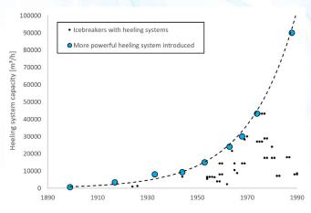
Through the 20th century, the capacity of active heeling systems increased rapidly with each new icebreaker generation and can be said to having reached its ultimate development with the 1988-built Swedish icebreaker *Oden*.
