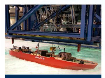
In addition to unbroken level ice, the effectiveness of the active heeling system was also evaluated in thick brash ice representing a large pressure ridge field.
