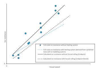
The calculation method was evaluated against data from the full-scale ice trials of the Finnish icebreaker *Otso*.
