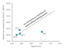
Results from ice model tests with heeling system (HC 0 without forced rolling; HC 1-3 with different system parameters).
