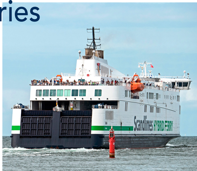
Scandline's 2016-built hybrid ro-ro ferry Berlin, which operates on the Rostock-Gedser route, features a 1.5-megawatt-hour (MWh) battery system. Photo source Pixabay
