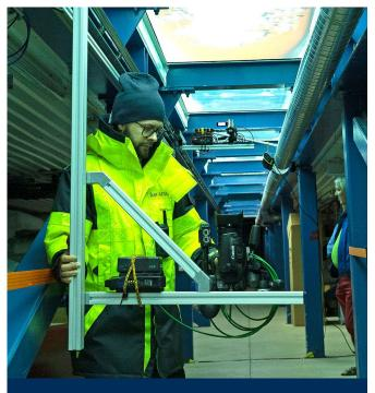
Shooting through the unique glass bottom in Aker Arctic's model testing basin, a recently-added fourth camera allows us to follow how both the bow and the rear of the model behave in ice. Toni Skogström manages the streaming.
