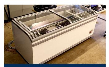
Ice-friction tests of hull coatings were performed last spring, and streamed online to both the customer and the Russian Register of Shipping (RS). The tests had to be performed at -20°C and Aker Arctic therefore developed a special measurement rig for the purpose, inspected and approved by RS.
