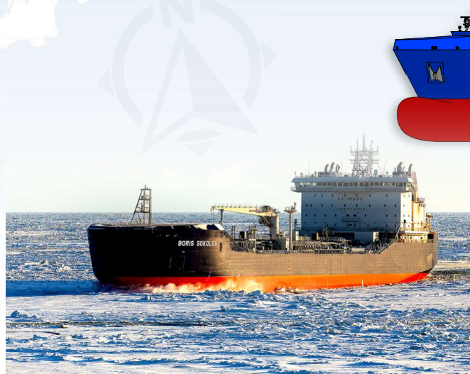
The Arctic condensate tanker Boris Sokolov has been delivering cargo from Sabetta to the markets since January 2019. The Arc7 ice class vessel is based on the Aker ARC 212 design and operates according to the Double-Acting Ship (DAS TM ) principle. Photo by Dmitry Lobusov
