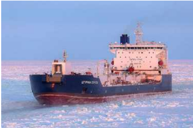
Shturman Skuratov is one of seven Arc7 shuttle tankers transporting crude oil year-round from Gazprom Neft's Arctic Gates oil terminal to Murmansk. The hull form was developed by Aker Arctic and its icebreaking performance was verified at our ice model test laboratory. Photo by Dmitry Lobusov
