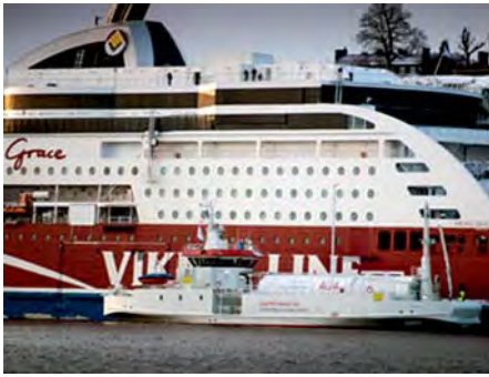
"Viking Grace" receiving LNG fuel from a bunkering ship (Photo: Karl Gabor)
