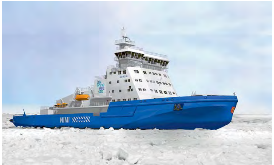
The new dual-fuelled icebreaker for the Finnish Transport Agency. The vessel is under construction at Arctech Helsinki shipyard and is due service at beginning of 2016. (Picture: Aker Arctic)
