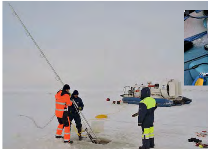
Lowering of sonar scanner under the level ice in front of the ice ridge.
