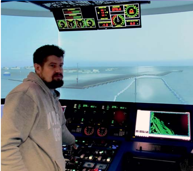
Yamal LNG Port of Sabetta feasibility studies, Captain Sampo Karppinen from ZPMC - Red Box Energy Services is steering. In the picture Captain Karppinen is reversing the Heavy Module Carrier in 1 m level ice and in the picture above right he is maneuvering the vessel to the quay in 3 m brash ice.
