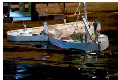
Pictures on the left: Seakeeping tests of the Trimaran concept, motions in waves with H_s = 4.0\text{m} , T_p = 9.0\text{s} and \varphi = 135^\circ
