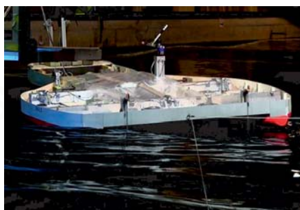
Seakeeping tests of the Trimaran concept, motion in waves with H_s = 4.0\text{m} , T_p = 9.0\text{s} and \varphi = 45^\circ
