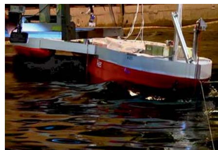
Seakeeping tests of the Trimaran concept, motion in waves with H_s = 4.0\text{m} , T_p = 9.0\text{s} and \varphi = 45^\circ
