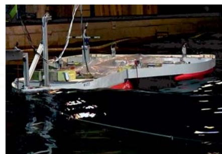
Seakeeping tests of the Trimaran concept, motion in waves with H_s = 4.0\text{m} , T_p = 9.0\text{s} and \varphi = 180^\circ
