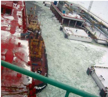
Example of flushing method using ice management vessel to clear the ice.
