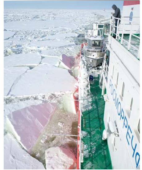
Baltika carried out the same operations as conventional icebreakers with just half of the propulsion power, as well as performed manoeuvres that are not possible for any other vessel currently in service.
