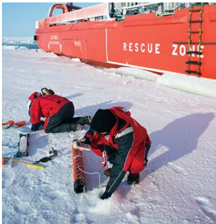
Teemu and Esko are measuring temperature and salinity profiles from core samples in order to determine the flexural strength of the ice.
