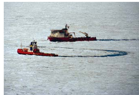
Icebreaker Smit Sakhalin cutting ice for CSO Constructor .
