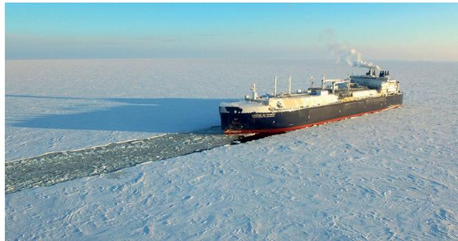
The first generation design of Arctic LNG carriers is extremely capable in ice and can sail independently through 2.1-metre-thick ice. The fifteen carriers, built to date, can manage on the NSR from July to December, whereas the second generation will manage year-round with a high transit speed through ice. In January 2021, three of the existing vessels undertook a test voyage along the NSR without icebreaker escort.
