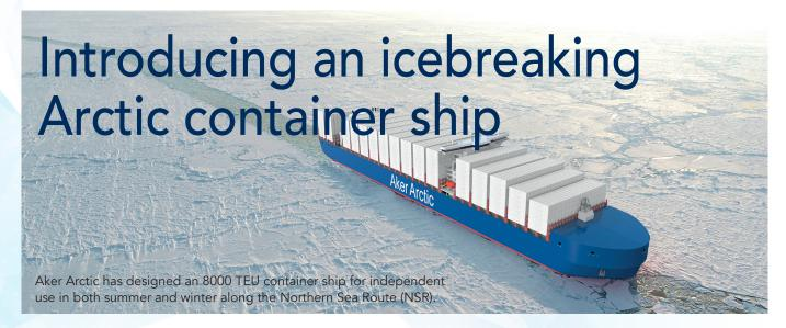
Aker Arctic has developed a completely new concept for the Northern Sea Route, an icebreaking Arctic container ship, which can be used year-round to cover the much shorter distance between Asia and Europe.
