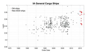
The length between perpendiculars (LPP) to overall length (LOA) ratio was closer to 1.0 for EEDI vessels, which indicates that many EEDI vessels have a very straight bow with a practically vertical stem in order to maximize the waterline length and improve efficiency in open-water.
