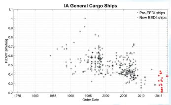
Ice class IA general cargo vessels are the most common cargo vessels in this environment. The new EEDI general cargo vessels have dropped their power-to-deadweight ratio by 30% compared to pre-EEDI vessels.
