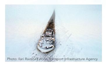
The totally new concept of a detachable icebreaking bow which is self-propelled and connected to the tugboat Calypso (pusher) during the winter season has been taken into use on Lake Saimaa, Finland's largest freshwater lake, and the Saimaa Canal.
