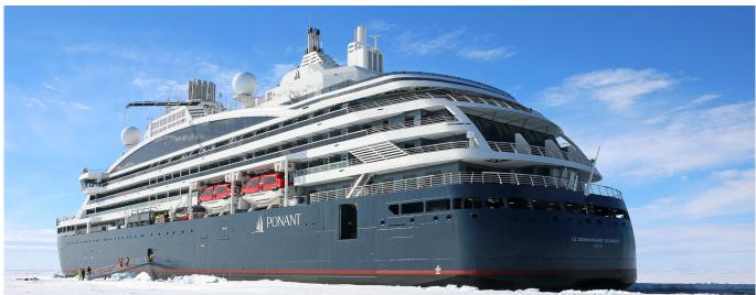
Le Commandant Charcot is designed according to the Double Acting Ship (DAS<sup>TM</sup>) principle which allows the vessel to operate both in ahead direction as well as stern-first, depending on the prevailing ice conditions.
